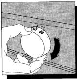
Following indications given in the drying times chart, turn the selector dial clockwise on the 60 mins setting of the blue section (Low Temperature Range).
